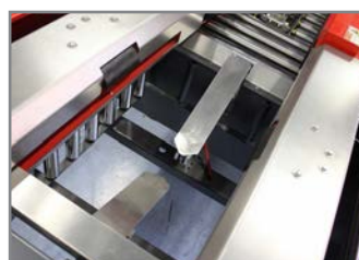
SISTEMA CHIUDI FALDE FLAP CLOSING SYSTEM
