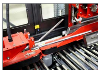
SISTEMA CHIUDIFALDE FLAP CLOSING SYSTEM
